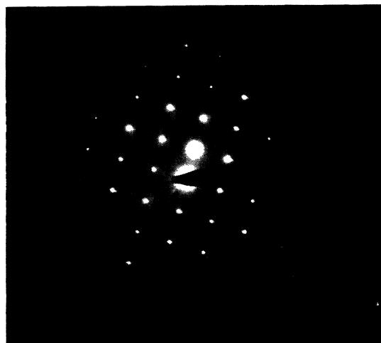
FIG. 3. Selected-area diffraction pattern of the 2223 phase reveals faint ringlike diffraction effects that surround some diffraction maxima. This pattern, which is consistent with the [21\bar{1}] zone axis, may result from point-defect clusters or other short-range ordering (Ref. 15).
