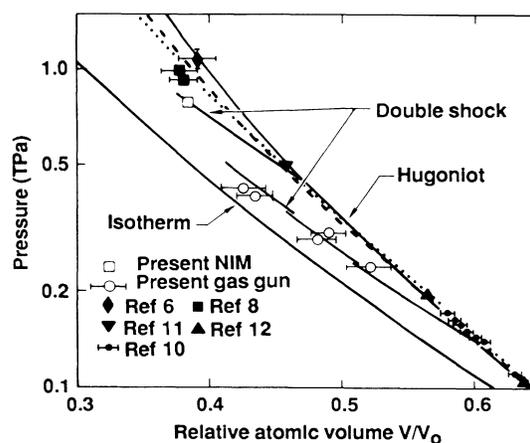
FIG. 1. Pressure-volume relations in Al. The filled and open circles are experimental single-shock (Hugoniot) and double-shock data, respectively, while the solid, dashed, and dotted curves represent the theoretical results derived from EOS 1, EOS 2, and EOS 3, respectively (1 TPa = 10 Mbar).
