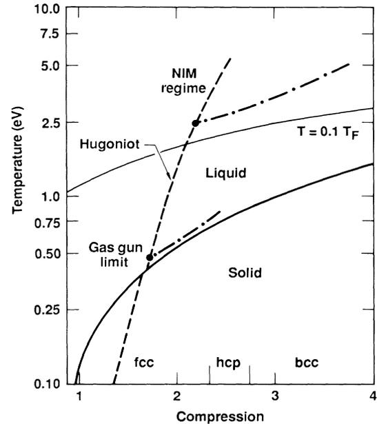
FIG. 3. Temperature along shock-compression curves in Al from EOS 1. The dot-dashed curves represent double-shock paths.
