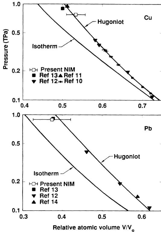
FIG. 2. Pressure-volume relations in Cu and Pb. The points are experimental Hugoniot data, while the solid curves represent the theoretical results derived from EOS 1.
