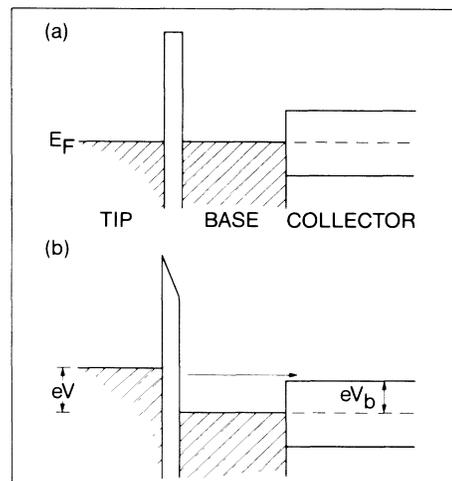
FIG. 1. Schematic energy-band diagram for the three-terminal BEEM experiment. The tunnel tip is separated by a vacuum barrier from the base metal. Terminals are applied to the tunnel tip, metal base, and semiconductor collector. Collector current  $I_c$  is measured between the base and collector. (a) The energy-band diagram for zero tunnel bias,  $V=0$ . (b) The energy-band diagram for tunnel bias greater than the barrier voltage,  $eV > eV_b$ .
