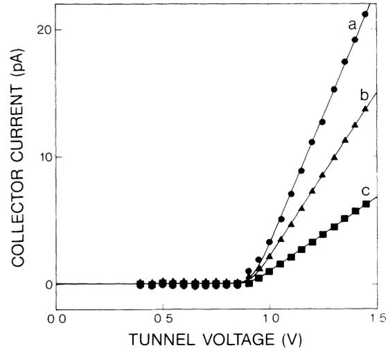
FIG. 2. BEEM spectroscopy results for the Au-Si heterojunction. BEEM spectra of collector current  $I_c$  vs tunnel voltage  $V$  are shown. Spectra *a* (dots), *b* (triangles), and *c* (squares) were measured at tunnel currents of 0.87, 0.57, and 0.27 nA, respectively. The calculated spectra (solid lines) correspond to barrier height values,  $eV_b$ , of 0.92 eV, and  $R$  values of 0.045, 0.045, and 0.043 eV<sup>-1</sup> for spectra *a*, *b*, and *c*, respectively.
