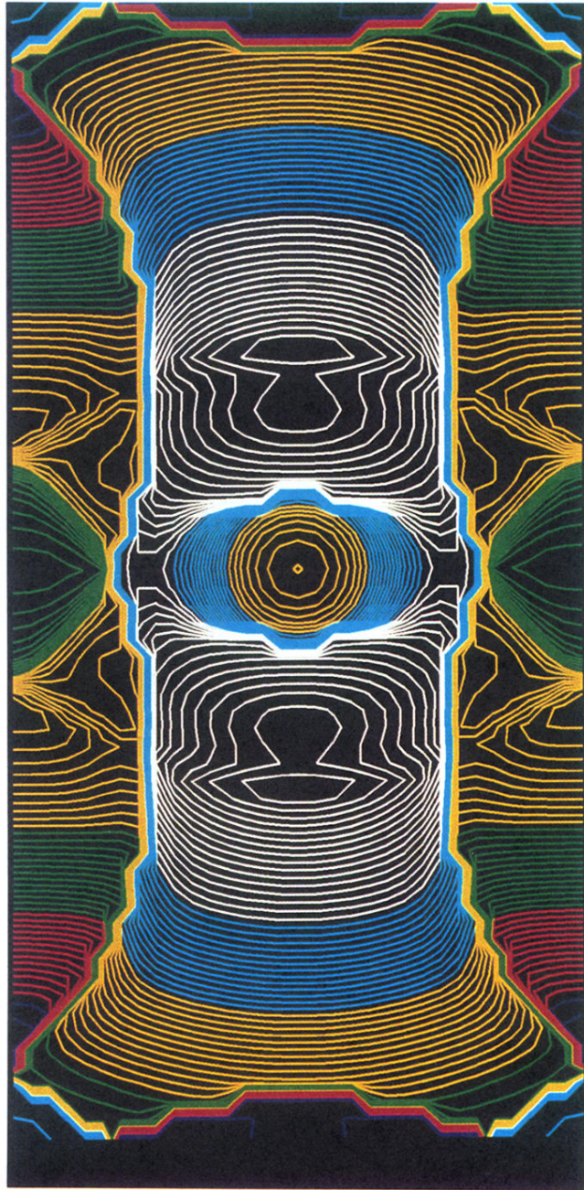
FIG. 4. The contour plots of the force experienced by the tip T_1 (held at \approx 2 \text{ \AA} above the surface) after the complete relaxation of the surface due to the tip's presence at each surface ( xy ) site. Contours in white show the repulsive regime. Attractive force in the range of 0 to -0.83 is shown in turquoise, between -0.83 and -1.66 in yellow, between -1.66 and -2.49 in green, between -2.49 and -3.32 in red, and less than -3.32 in blue. All forces are in units of 10^{-9} \text{ N} .
