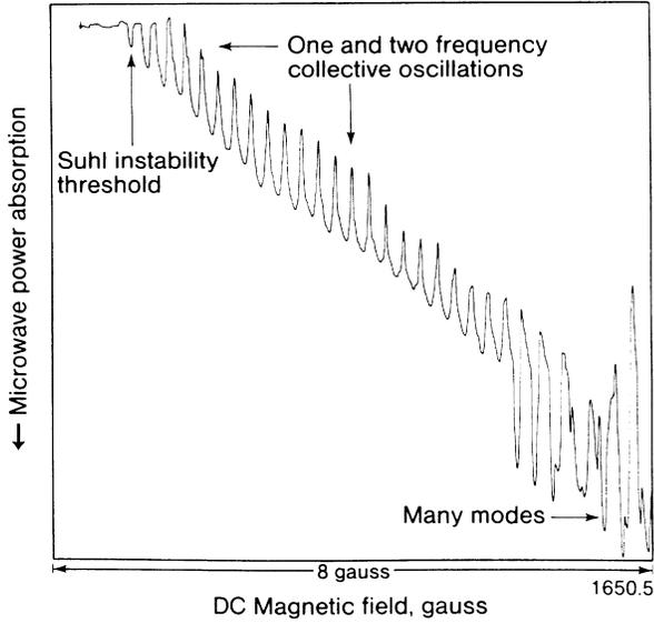
FIG. 2. Microwave absorption in an yttrium iron garnet sphere as the magnetic field is increased through the Suhl threshold, showing sequence of single spatial spin-wave modes, spaced by  $\Delta H_0 \approx 0.157$  G.
