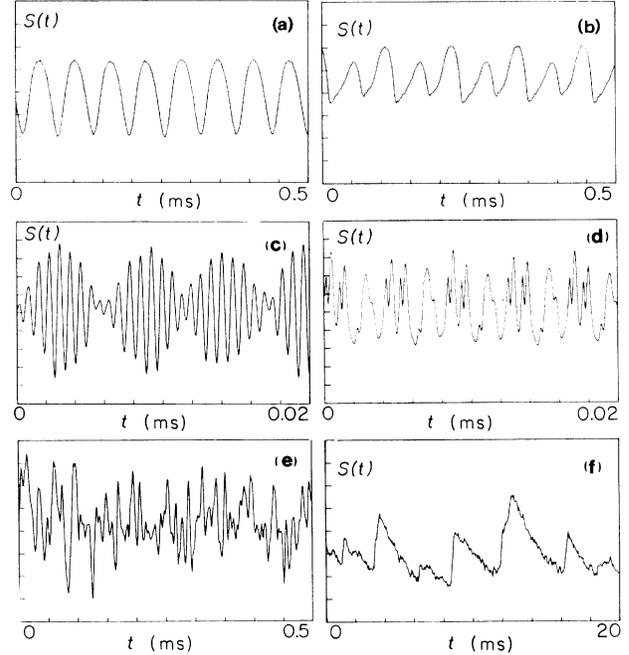
FIG. 3. Observed ac signals  $S(t)$  in spin-wave instability showing (a) periodic oscillation at 16 kHz; (b) period doubled; (c) quasiperiodic; (d) frequency locking; (e) chaotic; (f) aperiodic relaxation oscillation.
