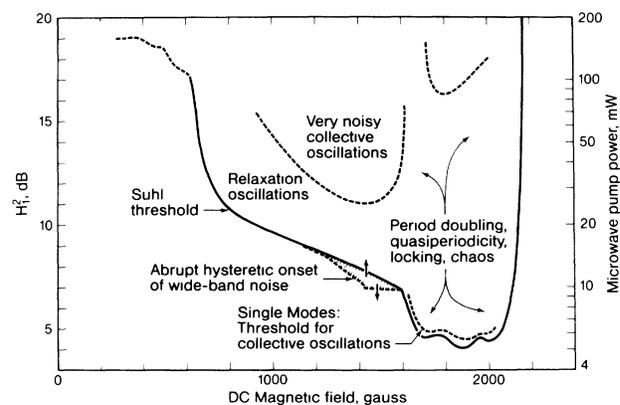
FIG. 1. Regions and boundaries of types of experimentally observed behavior in the perpendicular-pumped spin-wave instability in an yttrium iron garnet sphere; dc field  $H_0$  vs microwave pump power  $P_i \propto H_1^2$ .
