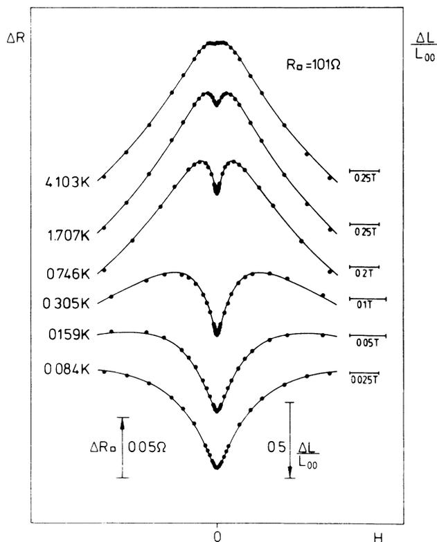
FIG. 1. Typical magnetoresistance curves of the Mg film covered by approximately 0.0022 atola of Fe. The field units are indicated at the right-hand side of each curve; the arrows give the scale for resistance and conductance changes. The points represent the experimental result; the curves are calculated with the Hikami-Larkin-Nagaoka theory.
