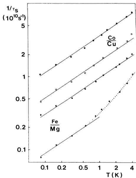
FIG. 3. Double-logarithmic plot of the temperature dependence of the magnetic scattering rates in the Mg/Fe films with about 0.0007 atola of Fe (open circles) and 0.0022 atola of Fe (filled circles), and the CuCo films with about 0.0025 atola of Co (open squares) and 0.007 atola of Co (filled squares), respectively. The slope of the solid lines is 0.50.
