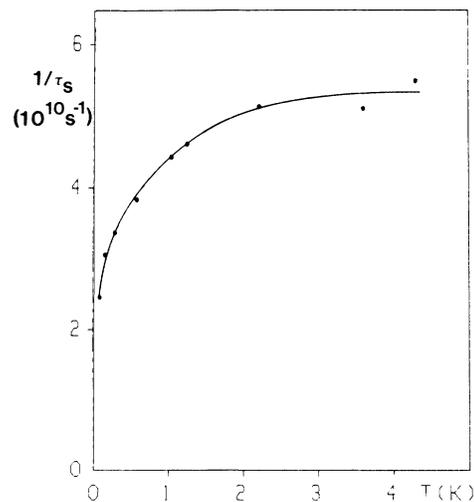
FIG. 2. Temperature dependence of the magnetic scattering rate in the Mg/Fe/Mg sandwich. The points show the measurements; the line is a guide for the eye.
