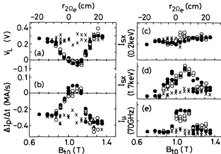
FIG. 4. (a) Loop voltage  $V_L$ , (b) ramp-up rate  $\Delta I_p/\Delta t$ , (c) SXR  $I_{sx}$  (0.2 keV), (d)  $I_{sx}$  (1.17 keV), and (e) ECE  $I_{\mu}$  (70 GHz) as functions of  $B_t$  ( $r=0$ ) or  $2\Omega_e$  EC resonance layer  $r(2\Omega_e)$ . Filled circles are for parallel injection of  $P_{EC}$ , open circles for antiparallel injection, and crosses for OH plasma.
