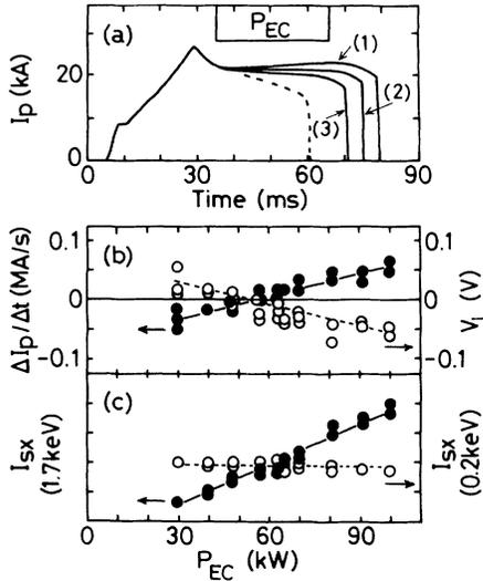
FIG. 3. (a)  $2\Omega_e$  EC-driven current ramp-up, flat-top, and ramp-down discharge for various  $P_{EC}$ : (1) 100 kW, (2) 57 kW, and (3) 30 kW. Dotted curve is without  $P_{EC}$ . (b) Ramp-up rate  $\Delta I_p/\Delta t$  (filled circles) and loop voltage  $V_L$  (open circles); (c) soft x-ray emissions  $I_{sx}$  (1.7 keV) (solid circles) and  $I_{sx}$  (0.2 keV) (open circles) as functions of  $P_{EC}$ .
