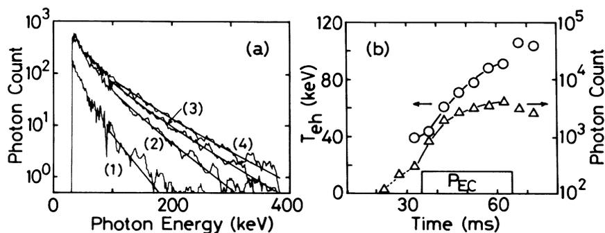
FIG. 2. (a) Energy spectra of hard x rays emitted from the plasma ( $P_{EC} = 100 \text{ kW}$ ,  $\tau = 30 \text{ ms}$ ,  $I_p \approx 25 \text{ kA}$ ) during time, (1)  $t = 30-35 \text{ ms}$  (OH plasma); (2)  $t = 40-45 \text{ ms}$  (ECCD plasma); (3)  $t = 50-55 \text{ ms}$ ; and (4)  $t = 60-65 \text{ ms}$ . (b) Temporal evolution of temperature of energetic electron tail,  $T_{eh}$  (circles) and photon count with  $h\nu > 92 \text{ keV}$  (triangles) as functions of time.
