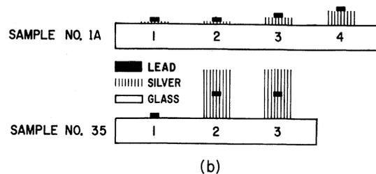
FIG. 1. (a) Critical current vs temperature for Ag-Pb samples of different geometry and silver thickness. The repeat data were obtained one week after the initial experiment. (b) Schematic cross section of the samples showing geometry and relative thickness. The critical current for sample 35-1 (pure lead) was 0.35 ampere, and was virtually independent of temperature.
