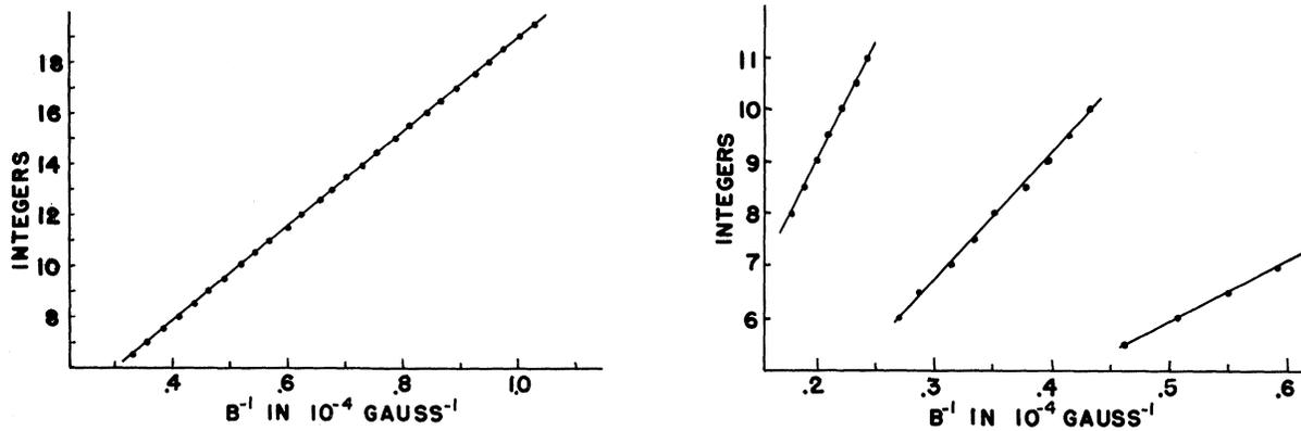
FIG. 2. Successive maxima and minima in  $dm/dt$  are plotted as integers and half integers vs  $B^{-1}$ , with  $n = 3.9 \times 10^{18}$  holes/cm<sup>3</sup> and  $T = 4.2^\circ\text{K}$ . (a) The plot for the longer period observed with  $\vec{B} \parallel \langle 100 \rangle$ . (b) The plots for all three periods observed with  $\vec{B} \parallel \langle 111 \rangle$ . Twenty-four more maxima and minima observed in the series with the smallest slope are not shown here.
