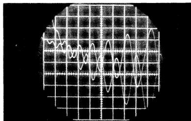
FIG. 1. dH-vA oscillations in *p*-type PbTe. The double trace shows the oscillations for increasing and decreasing magnetic field. The magnetic field varies from 7.3 kgauss at the left to 16.4 kgauss at the right.
