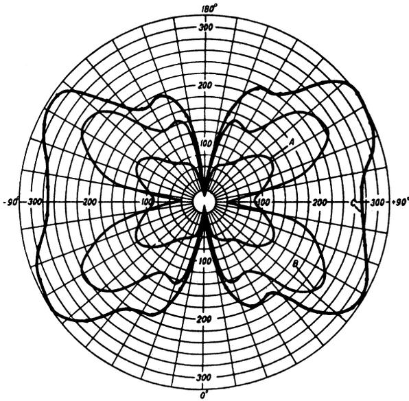
FIG. 2. Polar diagram of the transverse magnetoresistance,  $\Delta\rho_H/\rho_0$ , in Zn and Cd at 4.2°K.  $\alpha$  is the angle between the current  $J$  and the hexagonal axis, and  $r$  the resistance ratio,  $\rho_{273}/\rho_{4.2}$ , in zero field (after Justi et al.<sup>4</sup>).
