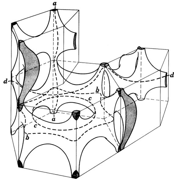
FIG. 1. The multiply-connected Fermi surface containing holes in the first Brillouin zone for Mg<sup>9</sup> (and probably Zn<sup>10</sup>), drawn in a periodically extended zone scheme. *aa*—open orbit along the hexagonal axis; *bb*, *cc*—closed orbits around the "ring"; *dd*—open orbit parallel to the basal plane.
