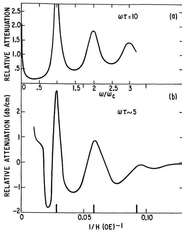
FIG. 2. (a) Predicted relative attenuation for ultrasonic cyclotron resonance after Cohen, Harrison, and Harrison.<sup>5</sup> (b) Observed curve in Ga single crystal derived from data in Fig. 1.
