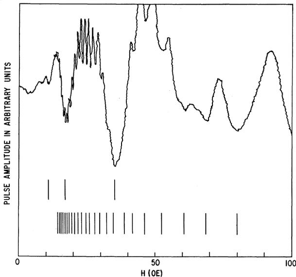
FIG. 1. Reflected ultrasound pulse in Ga as a function of magnetic field.  $f=115$  Mc/sec.  $T=1.5^\circ\text{K}$ . Upper reference marks indicate ultrasonic cyclotron resonance maxima. Lower reference marks indicate observed geometric resonance maxima.
