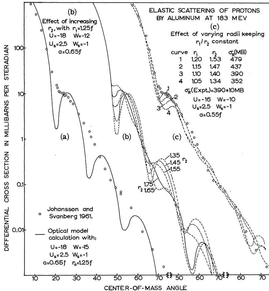
FIG. 1. (a) Experimental differential cross sections for the elastic scattering of 183-Mev protons by aluminum compared with an optical-model calculation with equal radii for the real and imaginary parts of the potential. (b) Calculated differential cross sections for the same interaction with increasing values for the radius of the absorbing potential. (c) The same for a series of radii, with  $r_2 = 1.27 r_1$ .
