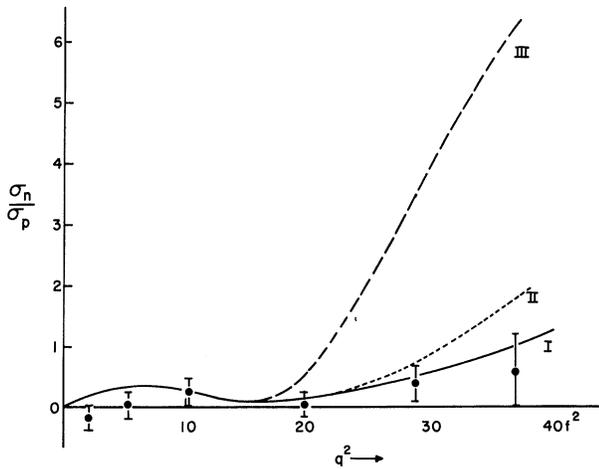
FIG. 3. The ratio of the neutron and proton cross sections as a function of the momentum transfer  $q$ . Curves I, II, and III were calculated with form factors  $F_{1p}$ , and  $F_{2p} = F_{2n}$  given by the curves I, II, and III in Fig. 2(a), and with  $F_{1n}$  from Fig. 2(b). The experimental points were computed from the data in Table I.
