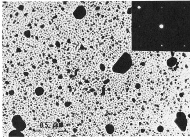
FIG. 1. Transmission-electron micrograph of Ag particles deposited on an amorphous  $\text{Al}_2\text{O}_3$  surface, prepared in the same manner as for completed tunnel structures. The average size of the smaller particles, which are numerically dominant in the picture, is comparable to the nominal film thickness of  $75 \text{ \AA}$  (magnification here is  $66 \times 10^3$ ). The inset shows a typical electron-diffraction pattern for the particles, indicating a crystalline structure.
