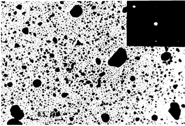
FIG. 1. Transmission-electron micrograph of Ag particles deposited on an amorphous  $\text{Al}_2\text{O}_3$  surface, prepared in the same manner as for completed tunnel structures. The average size of the smaller particles, which are numerically dominant in the picture, is comparable to the nominal film thickness of 75 Å (magnification here is  $66 \times 10^3$ ). The inset shows a typical electron-diffraction pattern for the particles, indicating a crystalline structure.
