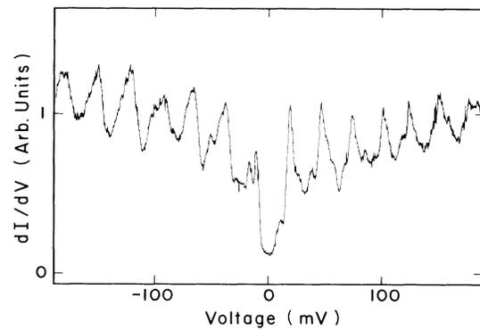
FIG. 3. Conductance trace ( $dI/dV$  vs  $V$ ) accentuating the structure shown in Fig. 2. Here we see, beginning at zero bias, the gap of  $e/2C$  in voltage, followed by a series of peaks separated by a voltage of  $e/C = 27$  mV. The latter are clear manifestation of the so-called Coulomb staircase expected for tunneling into particles with ultrasmall capacitance. The Ag particles accept a single additional electron each time a peak is passed.
