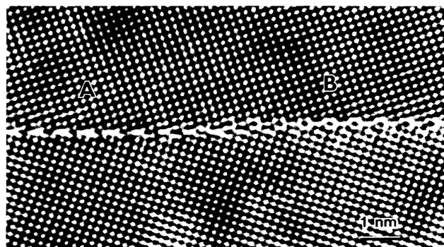
FIG. 1. Atomic resolution electron micrograph of a \langle 001 \rangle symmetric tilt grain boundary in NiO close to \Sigma=5 , (310), taken near optimum defocus (dark atomic columns). As the boundary translates from the left facet to the right one, the core structure changes from structure A to structure B.
