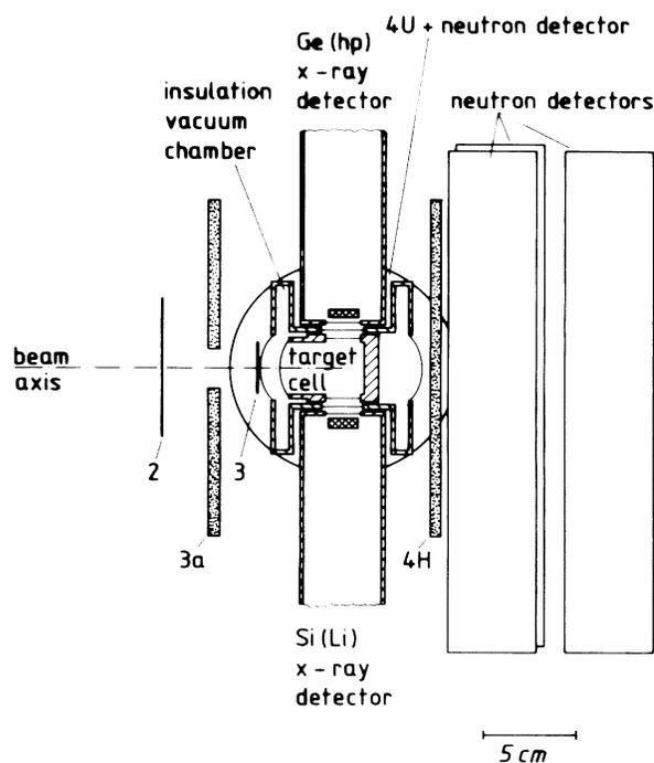
FIG. 1. Top view of the experimental setup for the  $dt$  experiment. Muons were detected with counters 2 and 3, electrons with counters 3a, 4U, 4H, and (not in the drawing) 4R and 4L.
