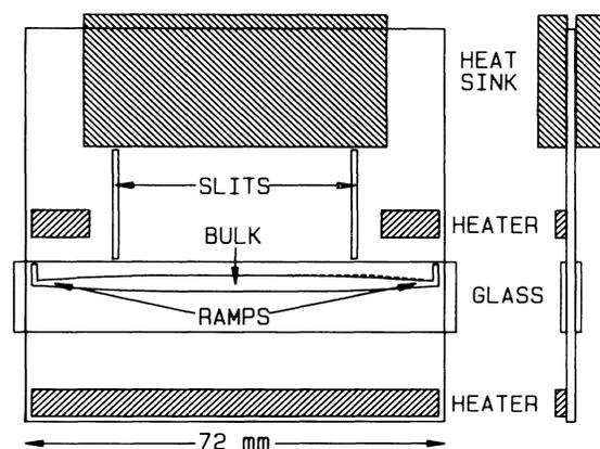
FIG. 1. The convection channel is cut out of a copper plate of  $72 \times 72 \times 1.5$  mm<sup>3</sup>. The dashed line indicates the pinning center.
