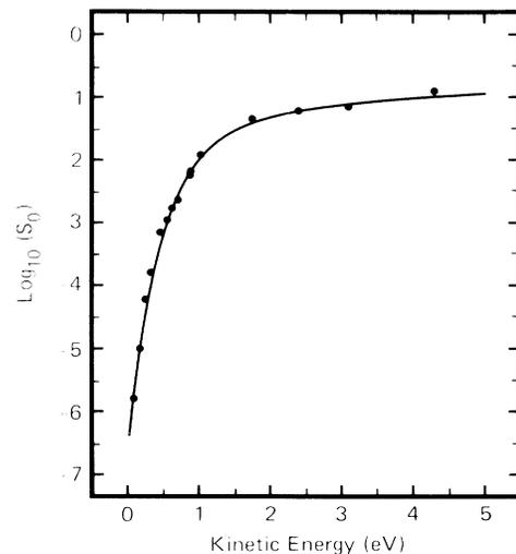
FIG. 1. Effect of incident energy on the dissociative chemisorption probability of  $N_2$  on Fe(111) at normal incidence and at a surface temperature of 520 K.
