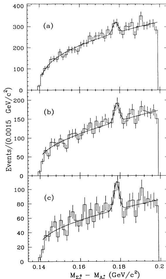
FIG. 2.  $M_{\Sigma_c^0} - M_{\Lambda_c^+}$  for several  $\Lambda_c$  minimum lifetime cuts: (a) no  $z_\gamma$  cut; (b)  $z_\gamma > 0.0 \text{ cm}$ ; (c)  $z_\gamma > 0.005 \text{ cm}$  (0.17 ps).
