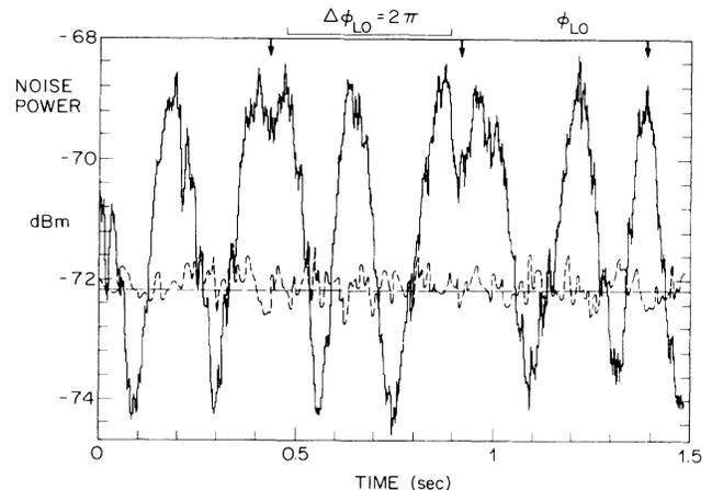
FIG. 2. Noise power at the output of the balanced detector, as a function of the local-oscillator phase. The dashed and solid lines correspond respectively to the squeezing cavity blocked and unblocked. The arrows on the  $\phi_{\text{LO}}$  axis indicate the reversals of the lead zirconate titanate (PZT) motion. The center frequency is 400 kHz, the rf bandwidth is 30 kHz, and the video bandwidth is 30 Hz.
