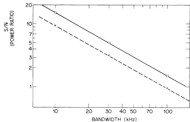
FIG. 4. Signal-to-noise power ratios as functions of the rf bandwidth. The dashed line corresponds to a vacuum input and the solid line to a squeezed-light input. These lines correspond to the expected  $1/B$  dependence. The open-circle and cross data points have been measured at 400 kHz, and the open-square and plus-sign data points at 850 kHz. These results illustrate the improvement in response time of the interferometer due to the use of squeezed light.
