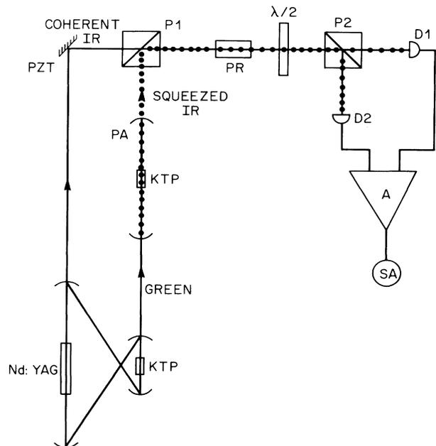
FIG. 1. Experimental setup. Coherent ir light from the cw Nd-doped yttrium-aluminum-garnet laser (left) and squeezed light from the parametric amplifier PA (right) are injected into the two input ports of the polarization interferometer (top) formed by polarizing beam splitters P1 and P2. A rotation of the polarization axes due to a polarization rotator PR is measured by an imbalance in detector currents D1 and D2 on a spectrum analyzer SA.
