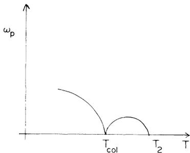
FIG. 2. Schematic behavior of the gap frequency (for the motion of the relative phase  $\theta = \theta_0 - \theta_2$ ) as a function of temperature. Near  $T_{\text{coll}}$ , the gap frequency goes to zero because of the cancellation of the restoring force.
