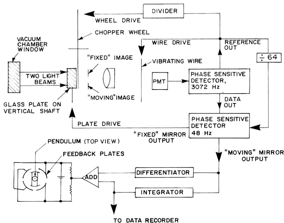
FIG. 1. Schematic diagram of the final stage of the optical detection system and the following electronics.
