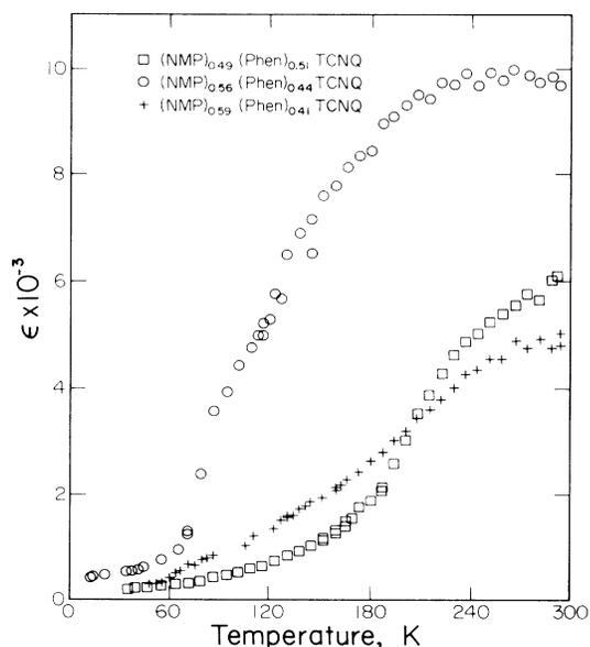
FIG. 1.  $\epsilon(T)$  at  $6.5 \times 10^9$  Hz for representative  $(\text{NMP})_x(\text{Phen})_{1-x}(\text{TCNQ})$  compounds.
