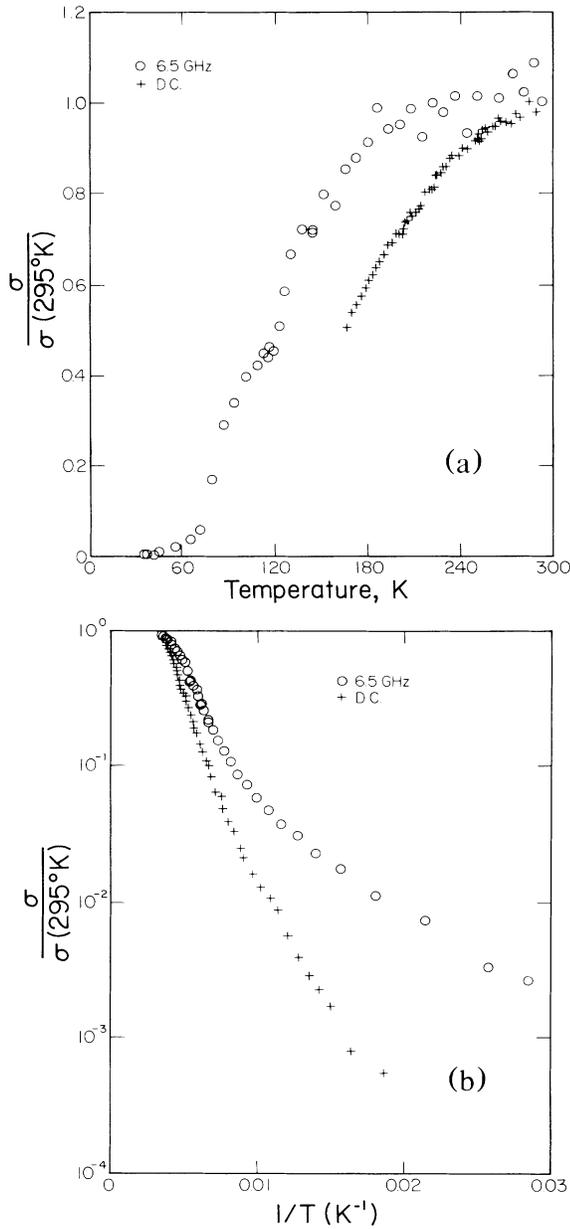
FIG. 3. dc and 6.5-GHz conductivity for representative  $(\text{NMP})_x(\text{Phen})_{1-x}(\text{TCNQ})$  samples. The microwave data are normalized to their dc counterparts. (a)  $\sigma$  vs  $T$ ,  $x=0.56$ ; (b)  $\log \sigma$  vs  $T^{-1}$ ,  $x=0.49$ .
