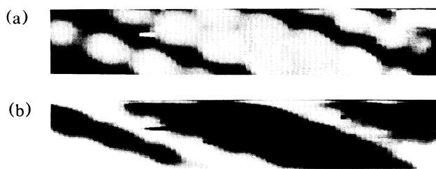
FIG. 4. (a) 64 \times 124-Å 2 constant-current topograph taken simultaneously with (b) a work-function image.
