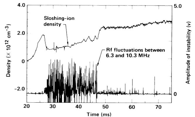
FIG. 2. The instability can cause large dumps of the sloshing ions. The sloshing-ion density is inferred from the charge-exchange flux measured by the  $45^\circ$  SED.
