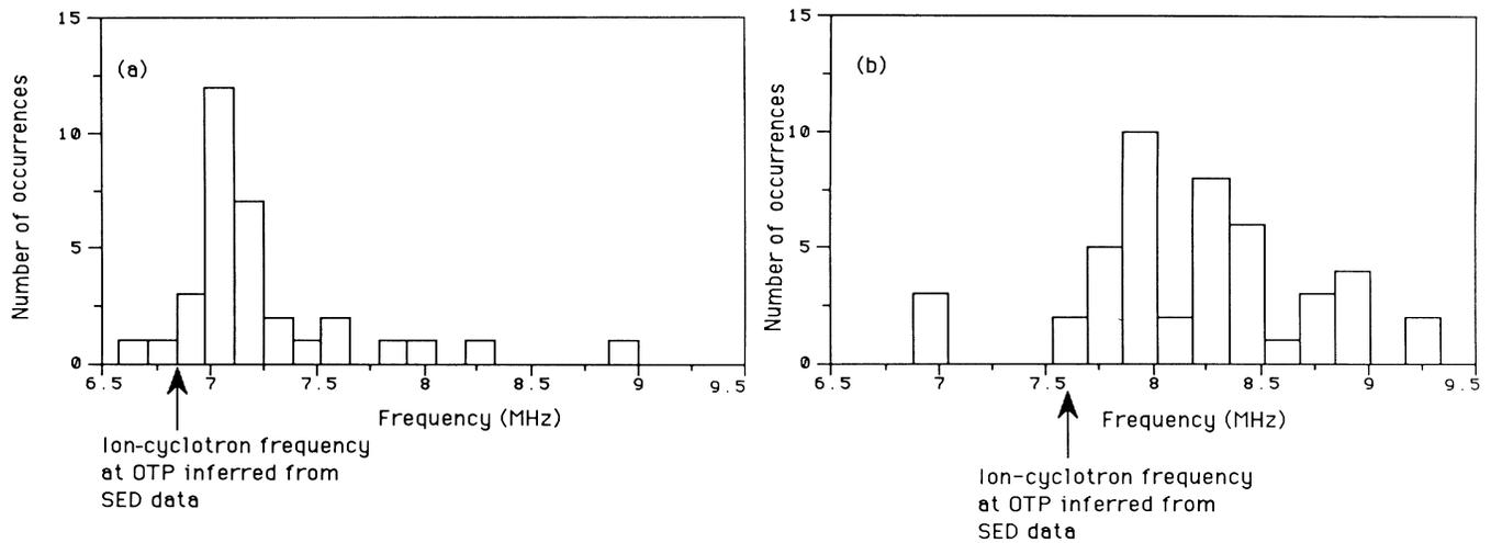
FIG. 1. Comparison of observed frequencies for shots (a) with  $47^\circ$  injection only and (b) with  $40^\circ$  injection or  $40^\circ$  and  $47^\circ$  injection.
