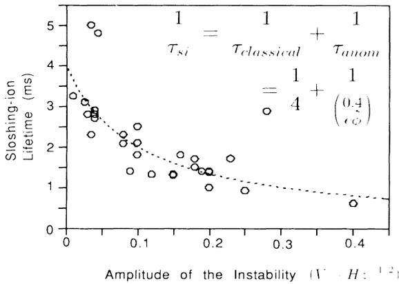
FIG. 3. The sloshing-ion lifetime depends on the amplitude of the instability. The sloshing-ion lifetime is determined from the sloshing-ion particle balance equation. For TMX-U parameters,  $\tau_s = [2.1I_{\text{beam}}(1.3n_{\text{total}}/n_{\text{si}} - 1)]^{-1}$ . Also plotted is the theoretical prediction of the sloshing-ion lifetime when a spectrum of fluctuations is present (Ref. 16). The anomalous lifetime is defined as
