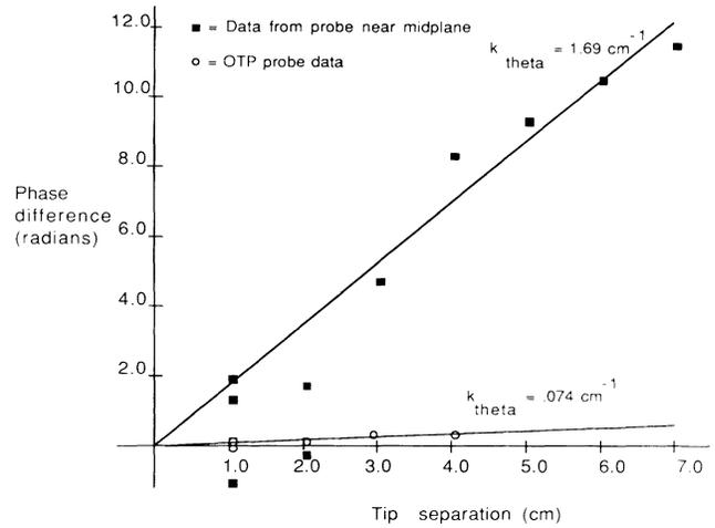
FIG. 4. Measured wavelengths near the midplane and outer turning point. These wavelengths have not been mapped back to the midplane.
