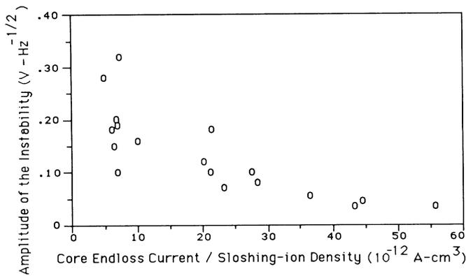
FIG. 5. The amplitude of the instability depends on the ratio of ion density in the loss cone to the sloshing-ion density. We take the core-ion end-loss current to be a measure of the density of ions in the loss cone.
