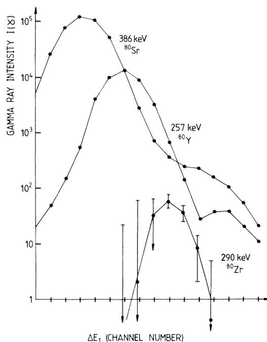
FIG. 1. Distribution of energy-loss signals  $\Delta E_1$  in the ion chamber for <sup>80</sup>Sr, <sup>80</sup>Y, and <sup>80</sup>Zr ions. The distributions were obtained by measurement of the intensity of coincident  $\gamma$ -ray photopeaks in spectra gated by energy loss.
