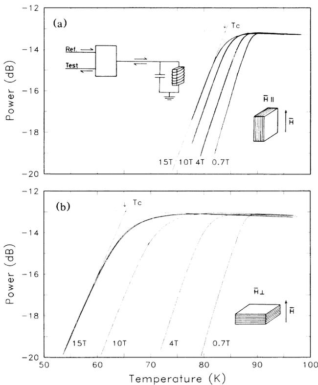
FIG. 1. Temperature dependence of the amplitude of the reflected signal from a resonant tank circuit with the  $Y_1Ba_2Cu_3O_{7-x}$  crystal mounted with the Cu-O planes (a) parallel and (b) perpendicular to the applied field, for  $H = 0.7, 4, 10,$  and  $15$  T. The constructions indicate how  $T_c$  at a given field was determined. Inset in (a): Schematic of the measurement apparatus.
