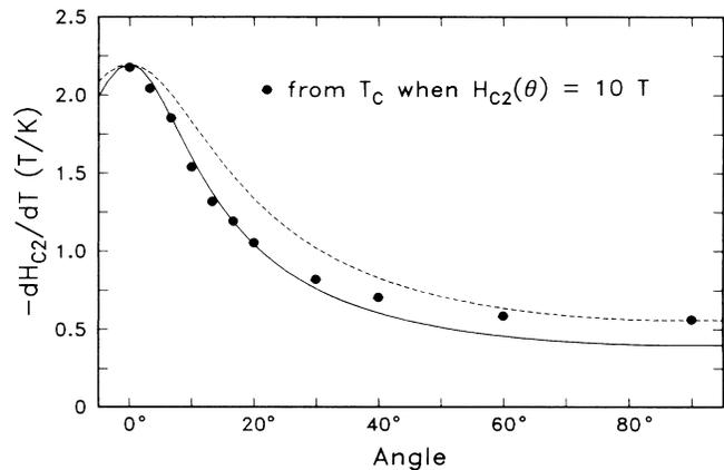
FIG. 3. Dependence of  $dH_{c2}/dT$  on angle between the Cu-O planes and the applied field as calculated from data taken at 10 T. The two curves are the angular dependences predicted by the anisotropic Ginzburg-Landau theory for two sets of anisotropy parameters.
