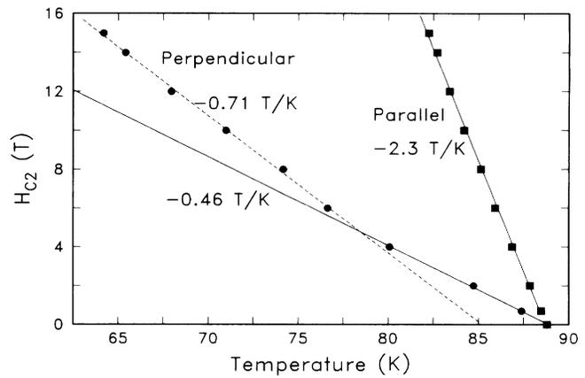
FIG. 2. Temperature dependence of the  $H_{c2}$  for the  $Y_1Ba_2Cu_3O_{7-x}$  crystal oriented with the Cu-O planes parallel and perpendicular to the applied field.
