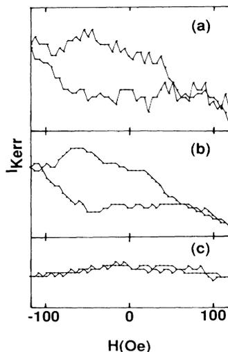
FIG. 3. (a) SMOKE ferromagnetic hysteresis loop at 460 K from three layers of Fe on (100) Cu grown at 460 K. (b) Average of eleven hysteresis loops on different runs from Fe films two and three layers thick, grown at 420 and 460 K and measured at  $\geq 360^\circ\text{C}$ . As shown in (c), the ferromagnetism disappears irreversibly upon cooling or after about an hour. (c) The eleven scans averaged after the ferromagnetism has disappeared.
