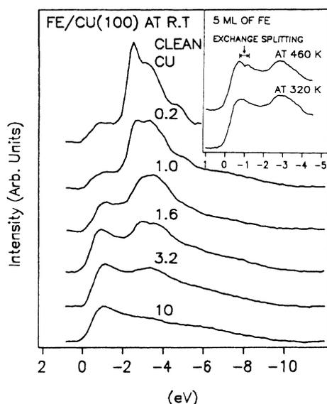
FIG. 1. Electron distribution curves showing relative number of electrons emitted (in arbitrary units) as a function of energy (in eV), relative to the Fermi energy, for iron on copper (100). The numbers indicate the number of monolayers (ML) of iron on copper (100). Inset: Energy distribution curves (EDC's) for five layers of fcc iron on Cu(100) at 460 K (top) and after cooling to 320 K (bottom).
