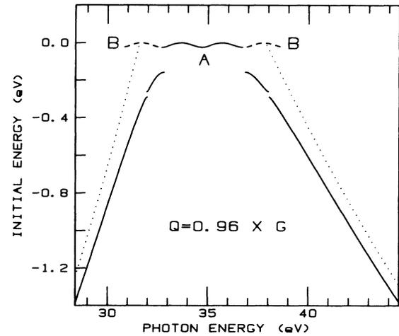
FIG. 1. Initial photoelectron energy vs photon energy for Na, from Ref. 3. The solid curve, for a CDW structure, shows emission in the gap (near *A*), where emission is not allowed in a (nearly) free-electron model, dotted curves. The dashed extensions at  $E_F$  (near *B*) are the "balcony" emission peaks allowed by the modified *k* conservation rule, Eq. (2).
