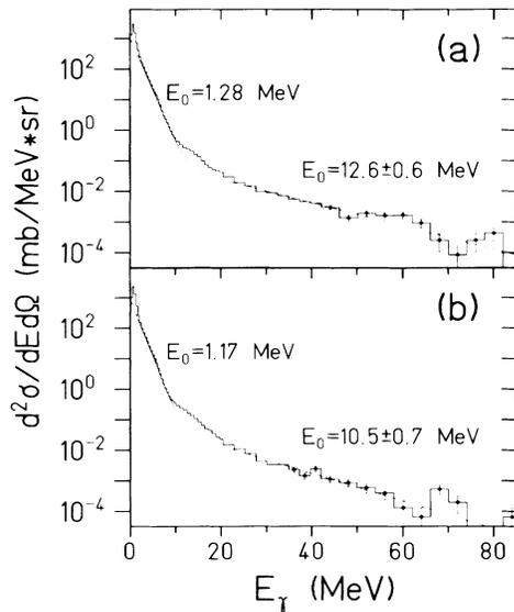
FIG. 1. Inclusive  $\gamma$ -ray spectra (a) at  $\theta_{\text{lab}}=90^\circ$ , and (b) at an average angle of  $\theta_{\text{lab}}=145^\circ$ . The solid curves represent fits with two exponential functions folded by the detector response.
