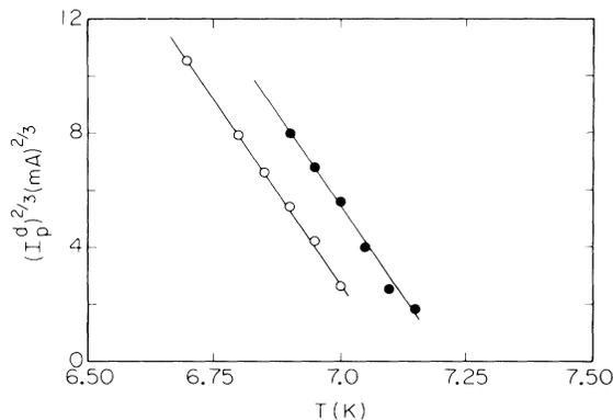
FIG. 3. Temperature dependence of the depinning current  $I_p^d$ .
