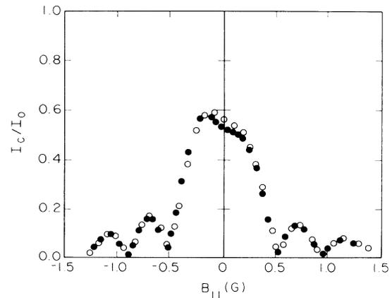
FIG. 2. Diffraction-pattern change for a small jump of the primary-only vortex in the  $x$  direction. Solid circles are for the vortex position  $(-0.59, 0.10)$  and open circles are for  $(-0.63, 0.10)$ .
