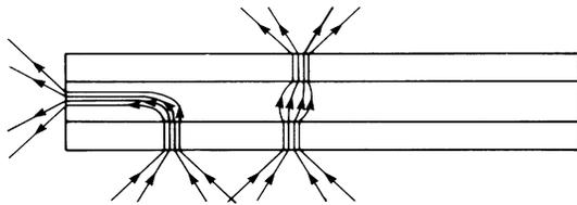
FIG. 1. Illustration of the vortex configuration trapped in the junction for  $B_{\perp\text{cool}}=0.016$  G. The misaligned primary-secondary vortex is shown near the center, and the primary-only vortex is sketched at the left.
