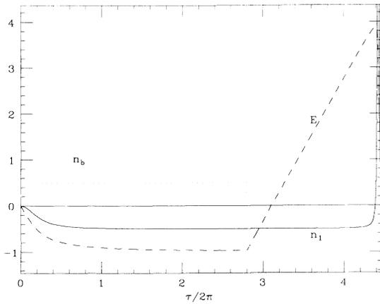
FIG. 1. Nonlinear plasma wave driven by beam of density  $n_0/2$ . Perturbed electron density, driving beam density, and electric field plotted as a function of  $\tau/2\pi$ . Densities are normalized to  $n_0$ ; electric field is normalized to  $m_e c \omega_p / e$ . For this case  $x_f = 16$ ,  $R = 4$ , and the maximum  $n_1/n_0 = 143$ .
