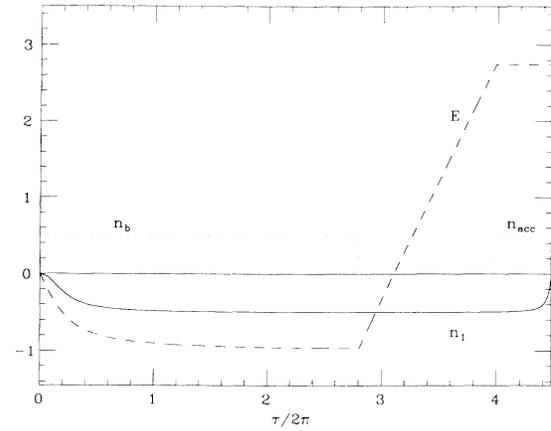
FIG. 2. Nonlinear plasma wave driven by beam of density  $n_0/2$ , with  $x_f = 16$ , loaded at constant electric field by accelerating beam with efficiency  $\eta = 0.5$ . Perturbed electron density, driving and accelerating beam density, and electric field plotted as a function of  $\tau/2\pi$ . Densities are normalized to  $n_0$ ; electric field is normalized to  $m_e c \omega_p / e$ .
