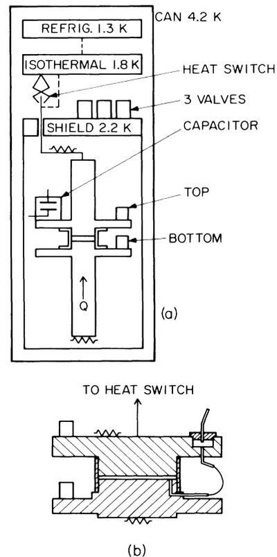
FIG. 1. (a) Schematic diagram of the cryostat showing cell K installed. (b) Cell J, shown in cross section.
