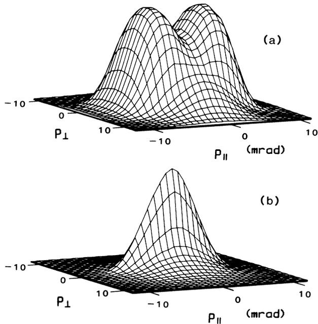
FIG. 1. 2D ACAR spectra for (a) HOPG and (b) C<sub>24</sub>K, at 100 K. Momenta  $\parallel$  ( $\perp$ ) to the  $c$  axis,  $p_{\parallel}$  ( $p_{\perp}$ ), in units of  $\text{mrad} \cong mc \times 10^{-3}$ . The 2D resolution is nearly a 2D Gaussian of  $\text{FWHM} \cong 1.4$  mrad. For clarity, lines are drawn only every 0.8 mrad, while data were taken every 0.4 mrad. The data are not symmetrized in either direction.
