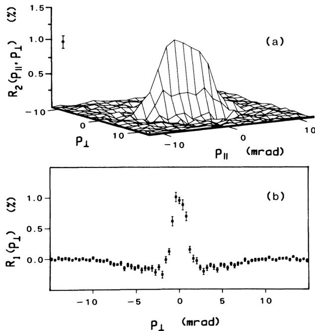
FIG. 3. Polarization effect for  $C_{24}K$  at 100 K as discussed in the text; (a) is obtained from 2D ACAR data, while (b) is the 1D equivalent. Momenta  $\parallel$  ( $\perp$ ) to the  $c$  axis,  $p_{\parallel}$  ( $p_{\perp}$ ), in units of  $\text{mrad} \cong mc \times 10^{-3}$ . The statistical uncertainty of the  $p_{\parallel}=0$ ,  $p_{\perp}=0$  point is shown on the left of (a).
