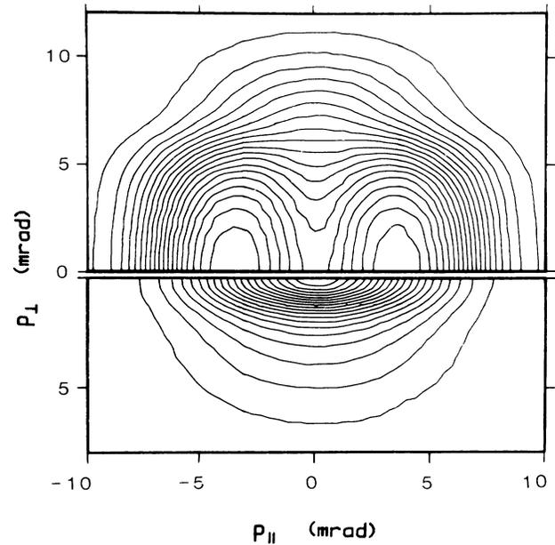
FIG. 2. Contour-line representation of half the 2D ACAR spectra of Fig. 1, for HOPG (top) and C<sub>24</sub>K (bottom). Momenta  $\parallel$  ( $\perp$ ) to the  $c$  axis,  $p_{\parallel}$  ( $p_{\perp}$ ), in units of  $\text{mrad} \cong mc \times 10^{-3}$ . Contours are equally spaced, in steps of 5%, from 5% to 95% of peak height for each sample.
