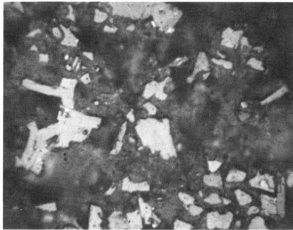
FIG. 1. Photomicrograph with reflecting optics of a polished section of the Y-Ba-Cu-O mixed-phase 93-K superconducting compound (Ref. 1). The white rectangular features are polished microcrystals of the opaque \text{YBa}_2\text{Cu}_3\text{O}_{6+x} phase. The horizontal dimension of the image is 150 \mu\text{m} .
