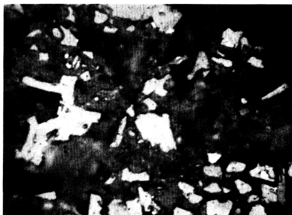
FIG. 1. Photomicrograph with reflecting optics of a polished section of the Y-Ba-Cu-O mixed-phase 93-K superconducting compound (Ref. 1). The white rectangular features are polished microcrystals of the opaque \text{YBa}_2\text{Cu}_3\text{O}_{6+x} phase. The horizontal dimension of the image is 150 \mu\text{m} .
