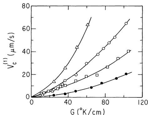
FIG. 4.  $v_c^{(1)}$  vs  $G$ . The open square, open circle, and open triangle represent samples of thickness  $d=19, 30, 50 \mu\text{m}$ , respectively. The closed circle is a  $30\text{-}\mu\text{m}$ -thick sample, to which hexachloroethane was added. The lines through the points are guides only.
