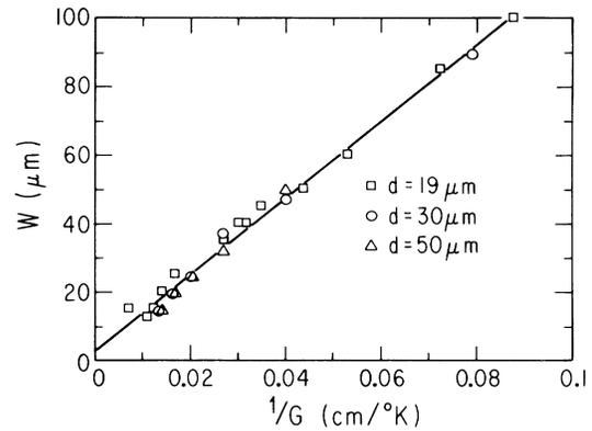
FIG. 2. Width  $w$  of the diffuse zone vs  $G^{-1}$  ( $d$  = thickness of sample).
