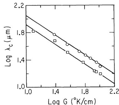
FIG. 5.  $\text{Log} \lambda_c$  vs  $\text{log} G$ .  $d=30 \mu\text{m}$ . Open square means 8CB alone; open circle means 8CB plus a small amount of hexachloroethane.
