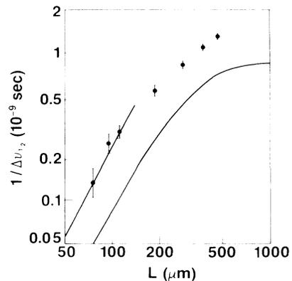
FIG. 4. Inverse of correlation frequency vs thickness, determined from average of autocorrelation function of intensity fluctuation. The solid curve is calculated from the theory in Ref. 16. The line through the data has slope  $m = 2$ .
