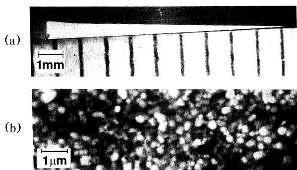
FIG. 1. Sample of  $\text{TiO}_2$  embedded in polystyrene. (a) Photograph of wedge. (b) Electron micrograph of sample.
