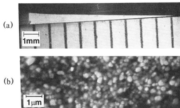
FIG. 1. Sample of TiO<sub>2</sub> embedded in polystyrene. (a) Photograph of wedge. (b) Electron micrograph of sample.
