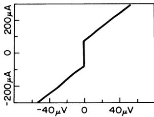
FIG. 1.  $I$ - $V$  characteristics of Nb/Ba-Y-Cu-O point-contact junction.
