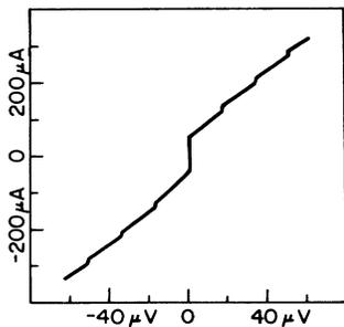
FIG. 2.  $I$ - $V$  characteristics of Nb/Ba-Y-Cu-O point-contact junction with the application of 8-GHz microwave radiation. Voltage steps can be clearly seen.
