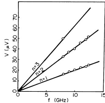
FIG. 3. Frequency dependence of the voltage steps. The lines give the slope  $n\Phi_0$ .
