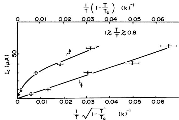
FIG. 4. Temperature dependence of the  $I_c$  of Nb/Ba-Y-Cu-O point-contact junction.  $I_c$  depends linearly on  $T^{-1}(1 - T/T_c)^{1/2}$ , where  $T_c$  is that of Nb.
