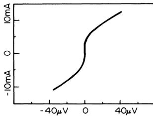
FIG. 5.  $I$ - $V$  characteristics of Ba-Y-Cu-O bulk sample just below its  $T_c$ .
