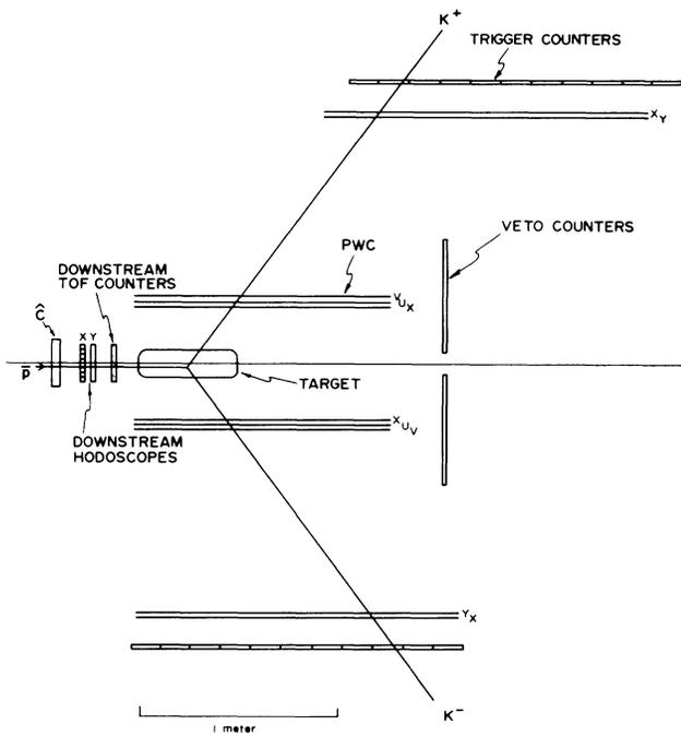
FIG. 1. Experimental arrangement.
