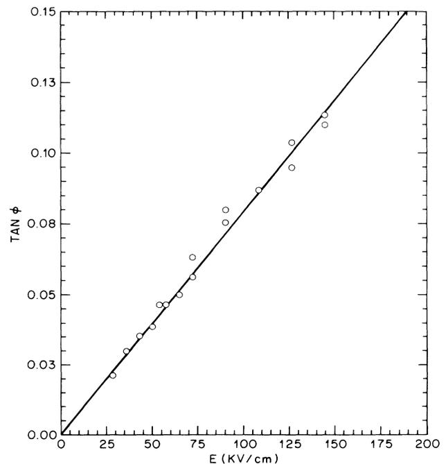
FIG. 1. Rotation of the optical axis ( $\tan\phi$ ) vs applied field ( $E$ ).
