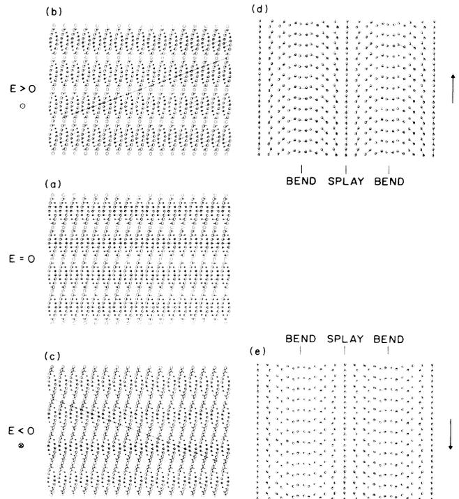
FIG. 2. The helical structure viewed normal to the helix axis, (a) in the absence of an electric field, and (b), (c) in the presence of an electric field perpendicular to the plane of the drawing, which shows the induced director rotation. (d), (e) Cross sections of the helix as indicated by the lines in (b) and (c), displaying the splay-bend pattern.
