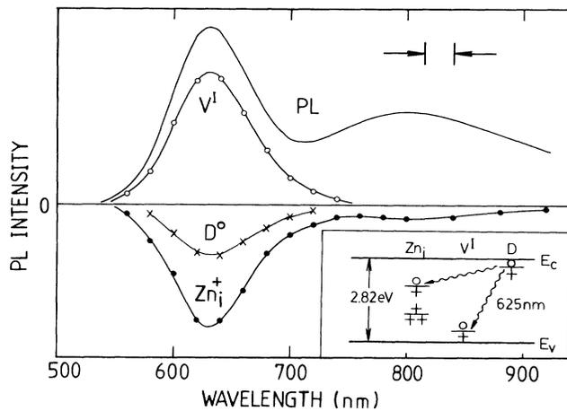
FIG. 1. Photoluminescence spectrum (PL) and spectral dependence of ODMR intensity for the Frenkel pair ( $V^I$ ), the distant shallow donor ( $D^0$ ), and the zinc interstitial ( $Zn_i^+$ ) for irradiated ZnSe at 1.5 K with 5 mW of 476-nm excitation. The inset illustrates the recombination processes involved in the ODMR detection.
