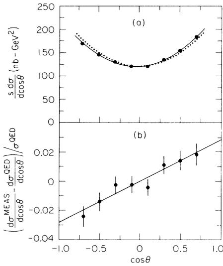
FIG. 1. (a) The measured differential cross section after efficiency and radiative corrections. The results of a one-parameter fit as described in the text are shown as the solid curve, together with the lowest-order QED cross section shown as the dotted curve. (b) The difference between the measured cross section and the QED cross section, divided by the total QED cross section. The solid line represents the fit to the angular distribution.
