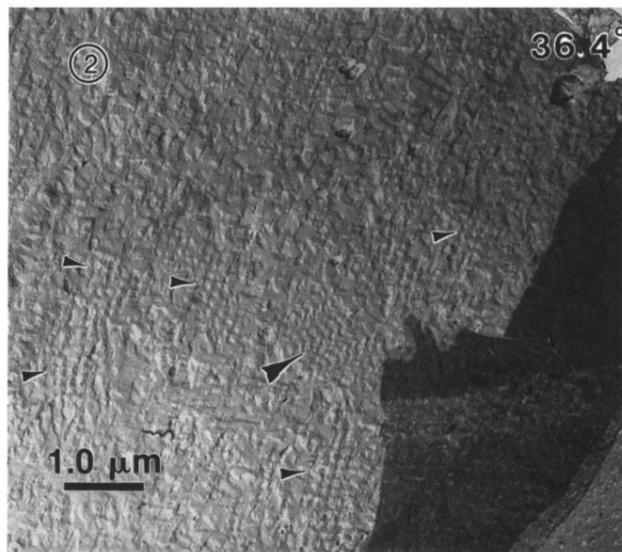
FIG. 2. As Fig. 1 except that CE4 was quenched from the BP I at 36.4°C. The small arrows point out square patterns along a {100} plane. The large arrow points toward a regular zigzag pattern. The two-dimensional periodicity is expected from the lattice structure of the BP I.
