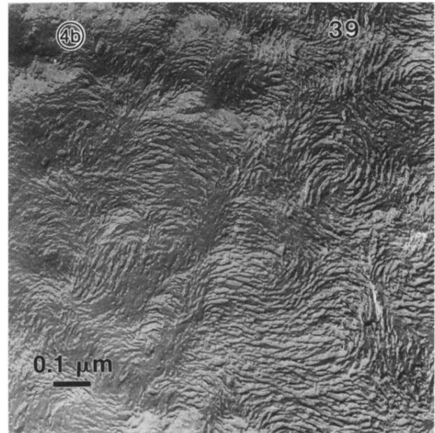
FIG. 4. (a) As Fig. 3(a), but nominally quenched from the isotropic at 38 °C. Slow initial cooling rates of the double-replica technique (see text) cannot trap CE4 as an isotropic liquid this close to the continuous transition from the isotropic to BP III. (b) As (a) except quenched from 39 °C. BP-III texture is observed. The isotropic to BP-III transition can only be avoided by starting the quench from  $> 45$  °C (see text).
