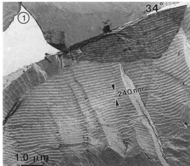
FIG. 1. Transmission-electron microscopy image of a freeze-fracture replica of CE4 (Ref. 9) quenched from the helical cholesteric at 34 °C to -190 °C. The pitch is 240 nm.
