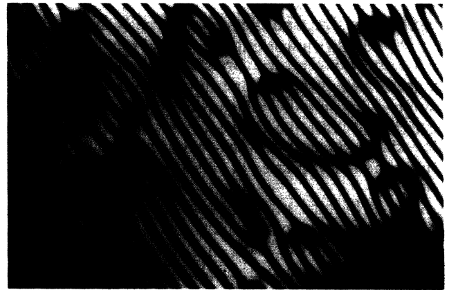
FIG. 1. Photomicrograph of periodic texture in a rotating sample of the N_L phase of potassium laurate-decanol- D_2O . The rotation axis is perpendicular to the stripes. The polarizer and analyzer are parallel to the short and long edges of the picture, respectively. The sample thickness d = 0.1 \text{ mm} , T = 19^\circ\text{C} , and the average spacing of the stripes \lambda_{cr} = 50 \mu\text{m} . H = 10 \text{ kG} .
