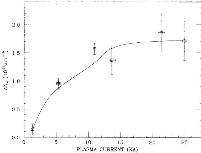
FIG. 4. Trapping efficiency ( $\Delta N_e$ ) shows strong correlation with plasma current.
