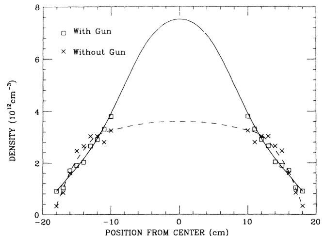
FIG. 3. Density profile found by use of Langmuir probe at edge and line-integrating interferometer.
