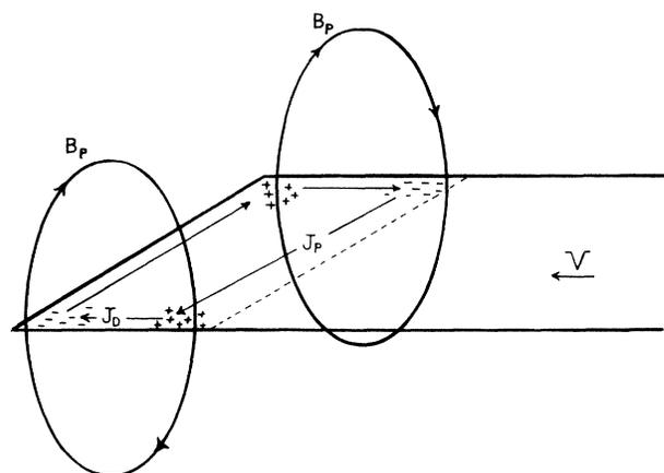
FIG. 1. Trapping mechanism for plasma injected into poloidal magnetic field. The polarization current ( $J_p$ ) provides a  $\mathbf{J} \times \mathbf{B}$  force with velocity  $\mathbf{V}$ . The depolarization current ( $J_D$ ), resulting from field reversal, drains charge buildup due to  $J_p$  and allows  $J_p$  to continue flowing until plasma is stopped.
