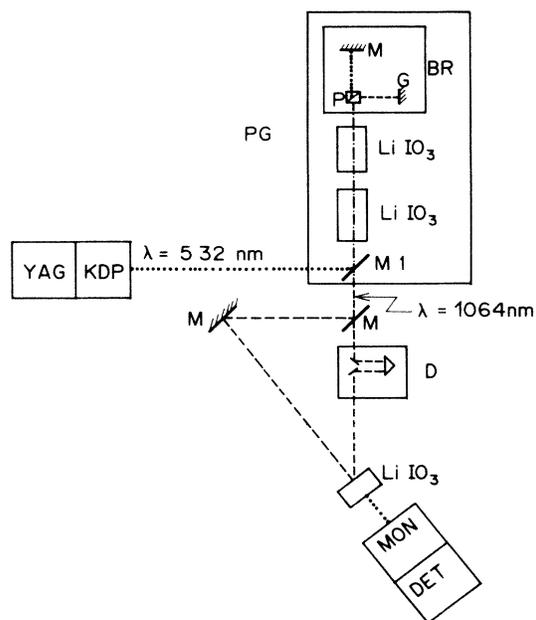
FIG. 1. Experimental setup (see text). PG, parametric generator; BR, backward reflector; P, Glan prism; G, grating; M, mirror; M1, dielectric mirror,  $R_{\max}$  at 532 nm; D, variable optical delay; MON, monochromator; DET, detection.
