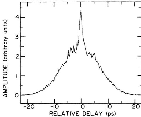
FIG. 3. Spectrally selected intensity autocorrelation of narrow-band degenerate parametric light. Narrow peak in center corresponds to twin-wave-packet correlation and follows the coherence profile of the pulses. Broad Gaussian corresponds to mixing uncorrelated wave packets and follows intensity autocorrelation profile of the pulses.
