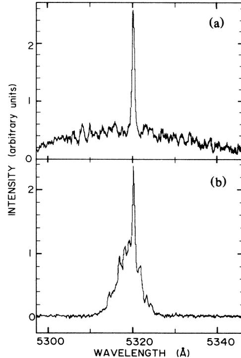
FIG. 2. Spectrum of frequency-doubled degenerate parametric light, averaged over 32 pulses: (a) Parametric generation with broad-band backward reflector, (b) parametric generation with frequency-dispersing backward reflector.
