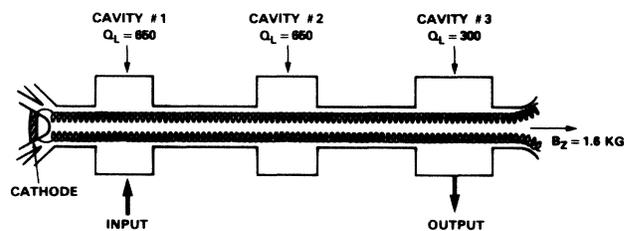
FIG. 1. Schematic of the three-cavity gyrokylystron configuration. The first two cavities are 6.06 cm in length while the third is 7.4 cm. The connecting drift spaces are 10.1 cm long.
