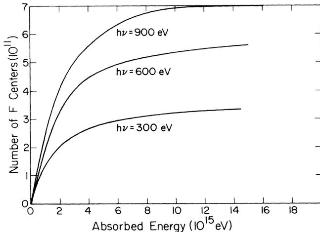
FIG. 2.  $F$ -center production near the surface of a KCl crystal as a function of adsorbed energy at x-ray photon energies of 300, 600, and 900 eV. The  $F$  centers are produced within an absorption depth ( $10^{-4}$ – $10^{-5}$  cm) very close to the surface and in an irradiated area of about  $2.0 \text{ mm} \times 1.5 \text{ mm}$ .
