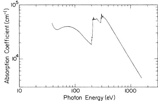
FIG. 3. Absorption coefficient of KCl as a function of photon energy. Data are from thin-film transmission measurements.
