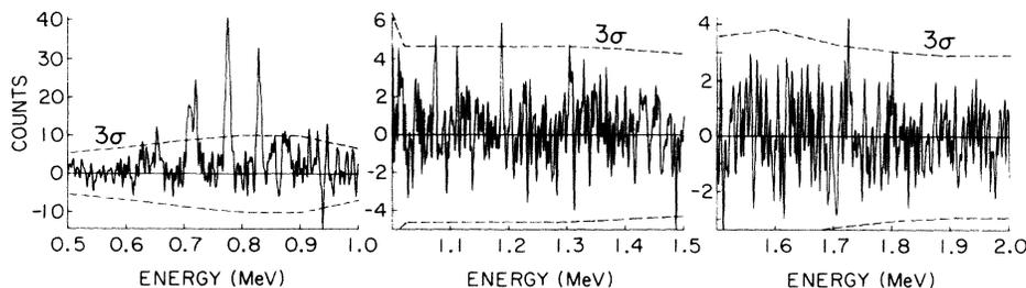
FIG. 3. Difference spectrum between Figs. 2(a) and 2(d). The dashed lines correspond to statistical 97% confidence limits (3 times the standard deviation) for a 4-keV-wide photon line. The expected  $\gamma\gamma$  line(s) should lie in the 1.5–1.8-MeV energy interval.
