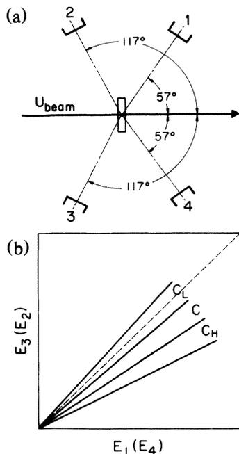
FIG. 1. (a) Experimental arrangement. The Th target is placed at  $90^\circ$  to the U beam. The Ge detectors (1-4) were placed 13 cm from the target at the angles shown. (b) Schematic sketch of the windows chosen to select the particular Doppler velocities: for  $C$ ,  $\beta = \beta_{c.m.}$ , for  $C_L$ ,  $\beta = 0$ , and for  $C_H$ ,  $\beta = 2\beta_{c.m.}$ . The photon energies are denoted by  $E_i$  where  $i$  is the detector number in (a).
