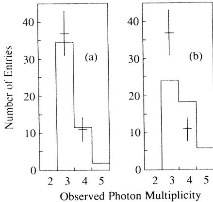
FIG. 2. Photon multiplicity in multiple-neutral-meson events. The points with error bars are the observed distribution, while the solid lines are the Monte Carlo predictions for (a)  $\tau^- \rightarrow \nu_\tau \pi^- \pi^0 \pi^0 \pi^0$  and (b)  $\tau^- \rightarrow \nu_\tau \pi^- \pi^0 \pi^0 \pi^0$  decay modes. The predicted distribution for the  $\tau^- \rightarrow \nu_\tau \pi^- \pi^0 \eta$  decay mode is nearly identical to distribution (b).
